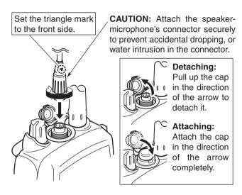
IMPORTANT: KEEP the transceiver's [SP MIC] connector cap attached when the speaker-microphone is not in use. Water will not get into the transceiver even if the cover is not attached; however, the terminals (pins) will become rusty, or the transceiver will function abnormally if the connector has become wet.
