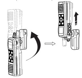
$\triangle$  Caution: Hold the transceiver tightly when hanging or detaching the transceiver from the belt clip.
